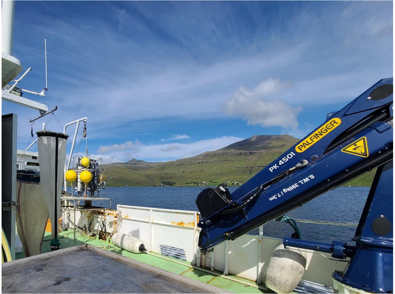
Figure 3.3 Fiskaaling research vessel. Niskin bottles in a rosette with an attached CTD (left) were used to sample water using the crane on board (right).
