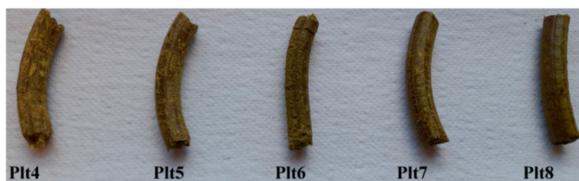
Figure 5. Five types of pellets composed of seaweed and wood chips.
