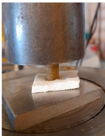
Figure 3. The sample in the compression test.
