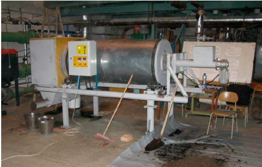
Figure 3.3- Steam-heater rotary dryer (Havlík & Dlouhý, 2020)
