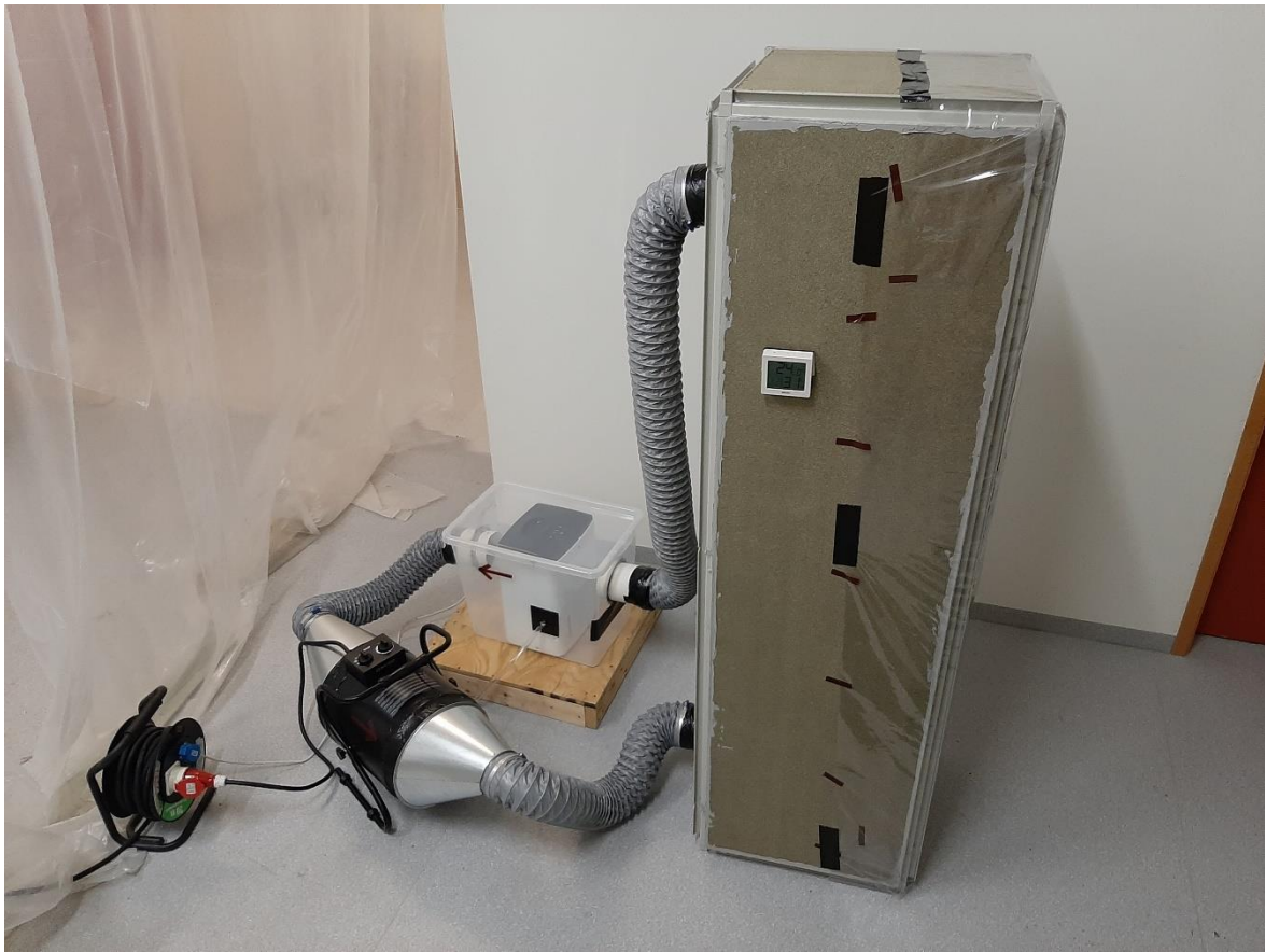
Figure 6.2- Prototype of the dryer with the heat recovery system
