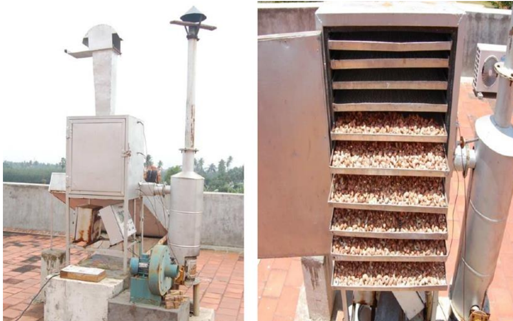
Figure 3.2- Cashew kernel dryer with biomass heater (Dhanushkodi, Wilson, & Sudhakar, 2015)
